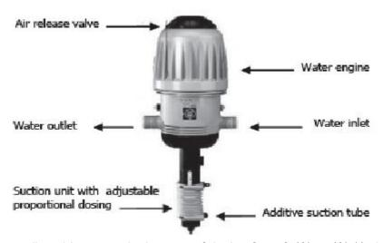
The pump has an adjustable proportioning rate of dosing from 0.4% to 4% (4mls to 40mls per litre water flow). The factory setting is 2% and can give up to 500 standard flushes from the 5 litre liquid enzyme container.
